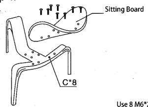
Use 8 M6\*25 screws to tighten the seat.
