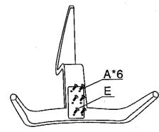
Use 6 M6\*15 screws to fix the iron sheet | Step 5: to the wooden frame.
