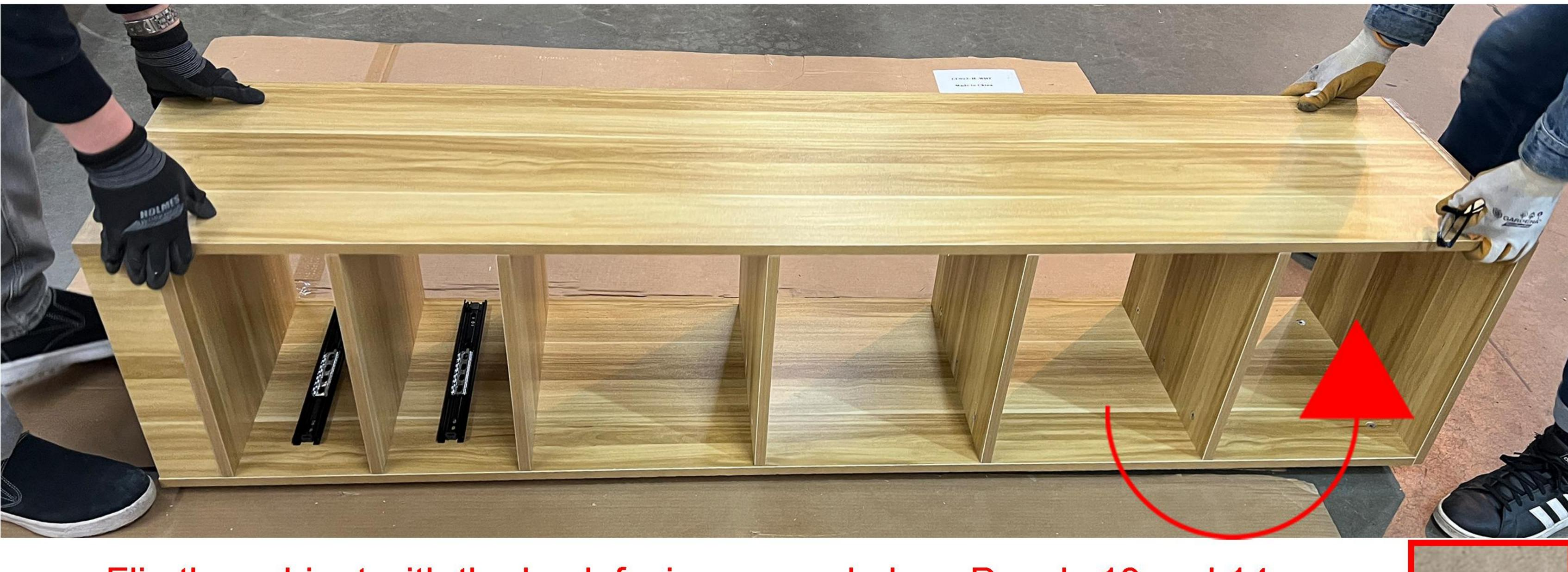
Flip the cabinet with the back facing up, and place Panels 13 and 14 on top. Use C to secure them to the frame.
