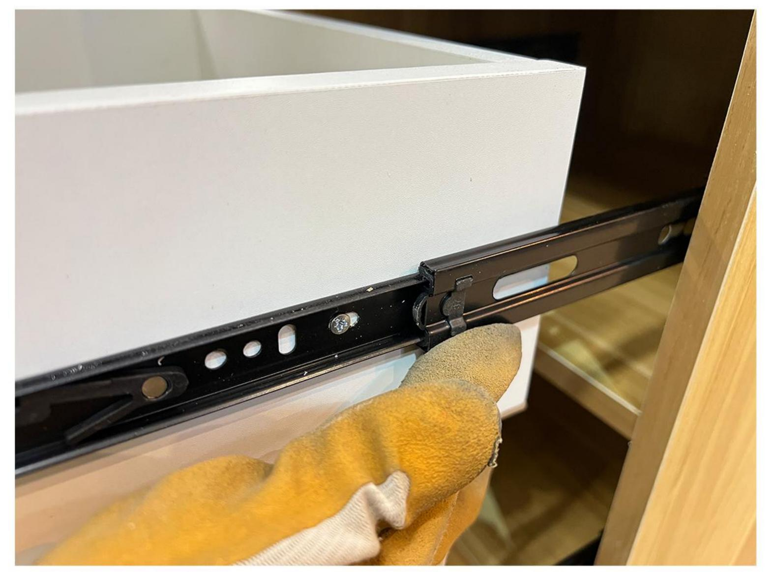
Insert the pull-out part of the sliding rail back into the main body part. Ensure both sides are properly aligned.
