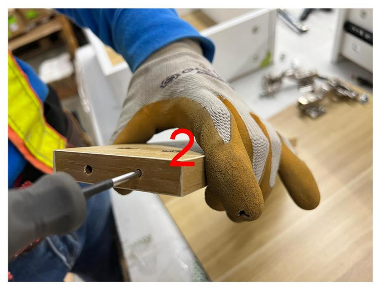
If the pre-drilled holes on the side of Panel 2 are not visible, you can use a screwdriver to pierce through the veneer and uncover the pre-drilled holes behind it.
