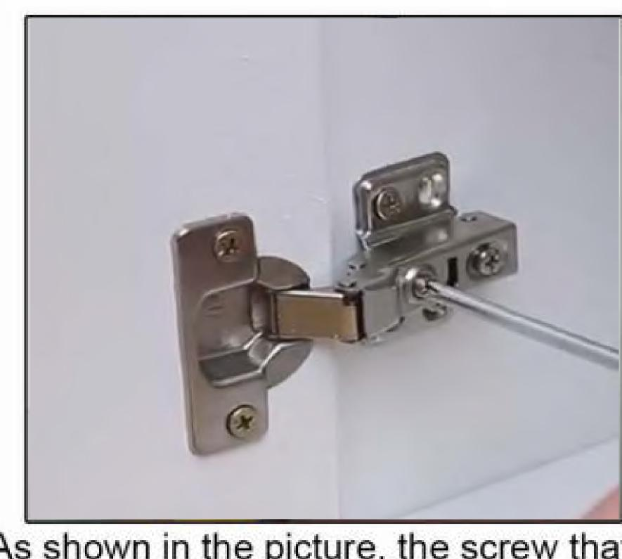
As shown in the picture, the screw that the screwdriver points to is used to adjust the door panel to move left and right, and turning it clockwise is to adjust the door panel to move toward the center.
