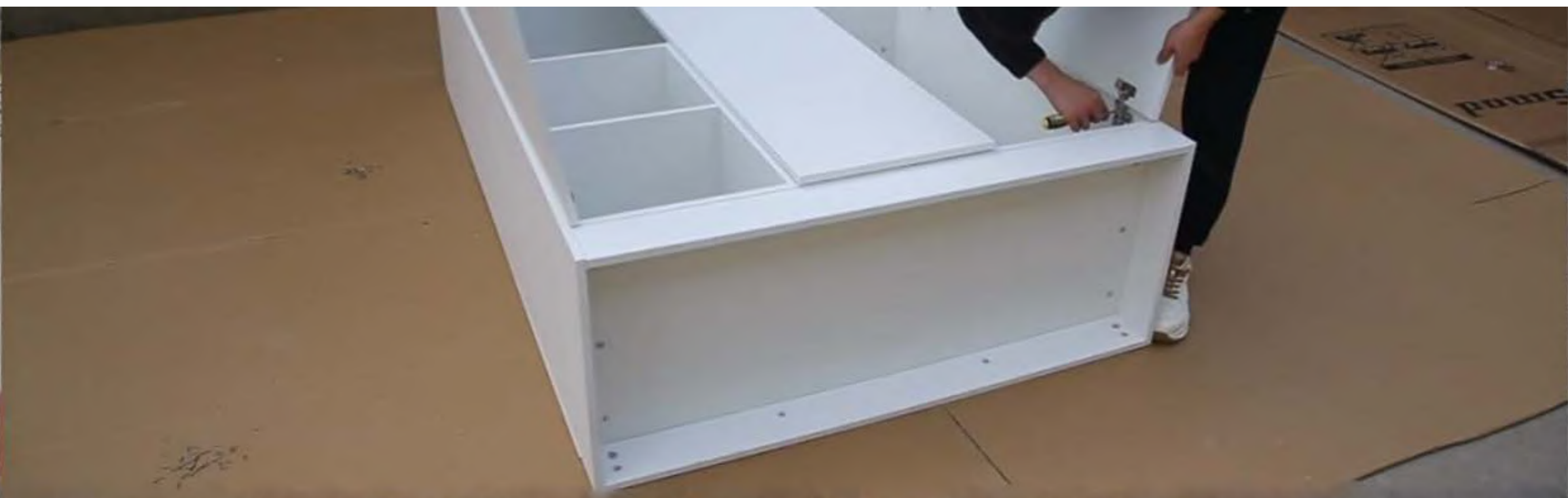
Install the cabinet door on the left and right side panels and the middle partition, and use self-tapping threads to fix the cabinet door hinges
